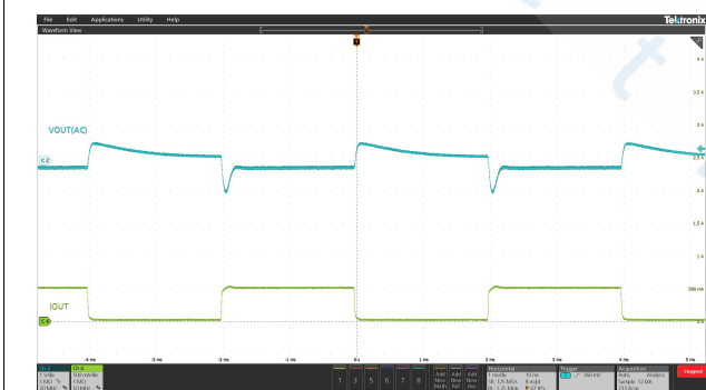
Figure 27. Shutdown Waveforms at Light Load
