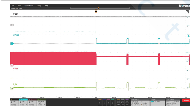
V_{DD} = 48\text{ V} , V_{OUT} = 12\text{ V} , I_{OUT} = 0\text{ A} to overload
